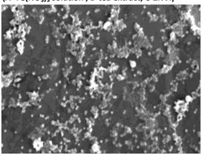
FIG 3: SEM image of the Starch stabilized nZVI
