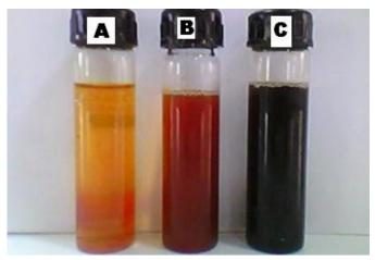
Fig 1: colour change during green ZNVI synthesis (A- Fe(NO<sub>3</sub>)<sub>3</sub> solution , B-tea extract, C-ZNVI)
