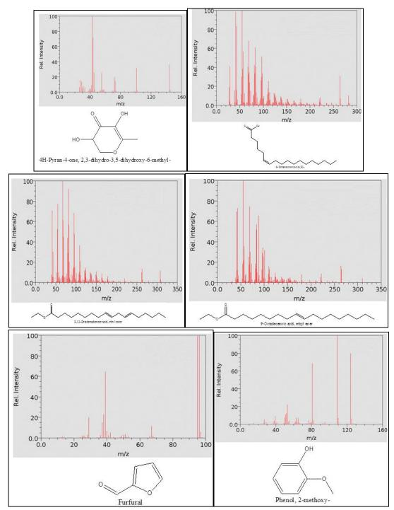
Figure 2: Mass fragmentation spectra and corresponding structures of the phytochemicals isolated from *Albizia lebbeck* root bark extract
